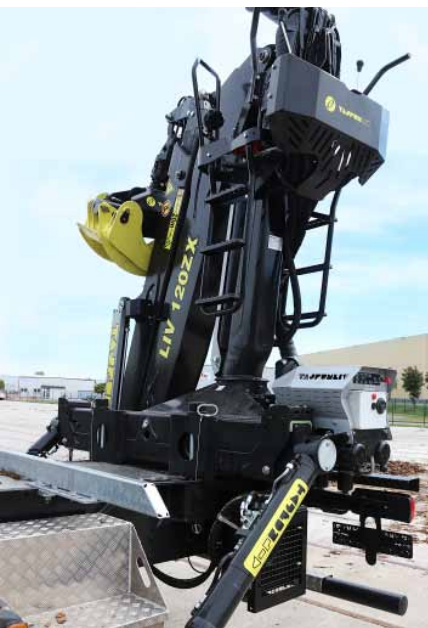
Despite the exterior hoses at the crane column, the LIV 120 ZX appears very orderly
