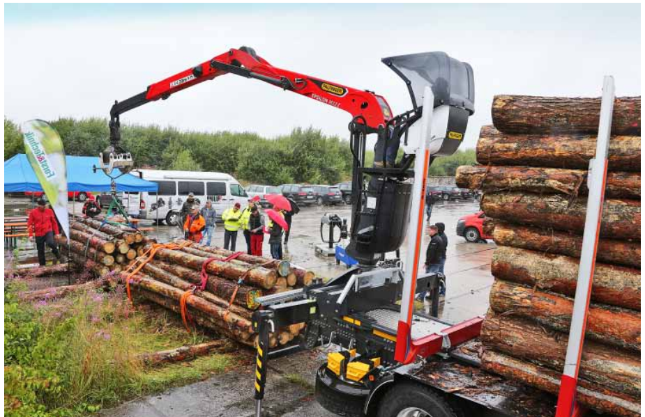
The lifting capacity was measured at three different outreaches: 3 m, 5 m and 7.5 m
