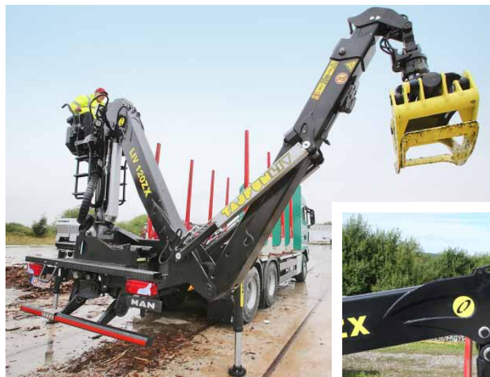
Despite the exterior hoses at the crane column, the LIV 120 ZX appears very orderly
