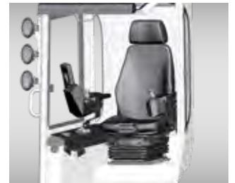
Convenient working position in air-suspended comfort seat
